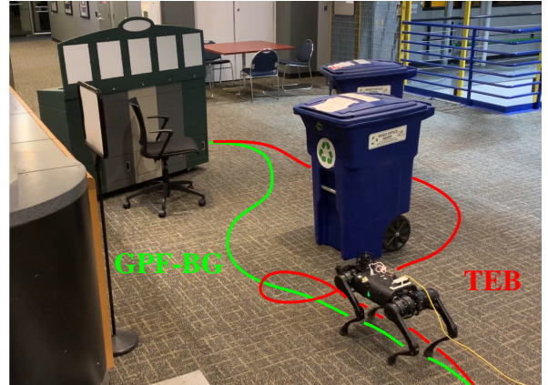
Fig. 7: The robot navigation paths for GPF-BG (green) and TEB (red) in a constrained environment.
