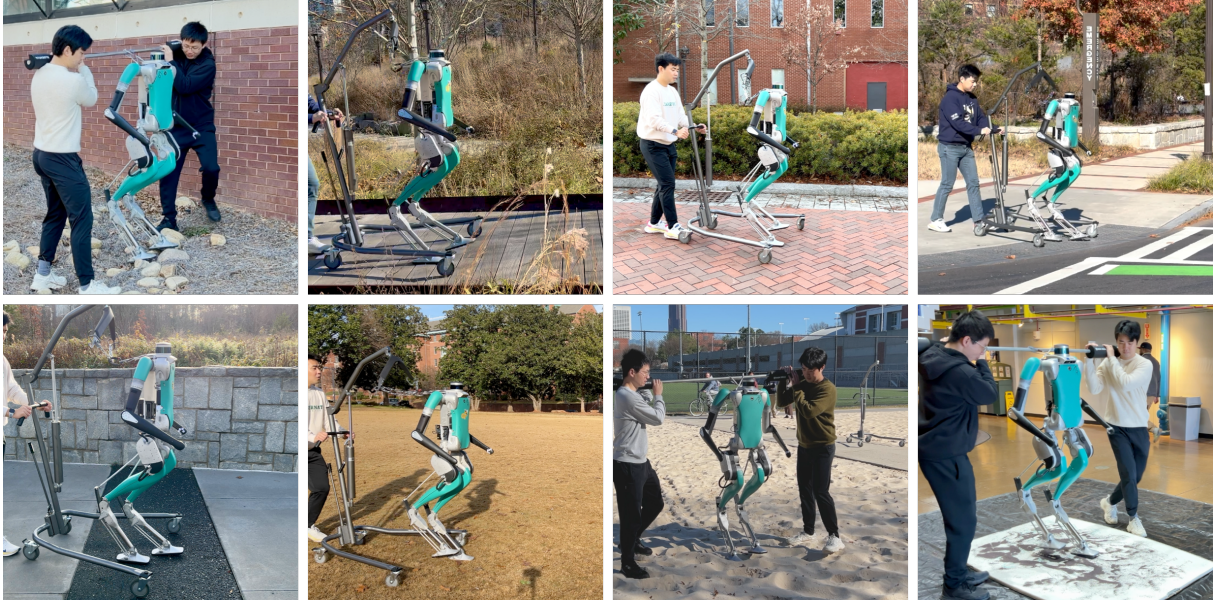
Fig. 1: We implement our L2T-RL algorithm on our bipedal walking robot Digit and deploy it on diverse terrain with various environmental conditions such as wet grass, gravel, sandy terrain, and slippery surfaces.
