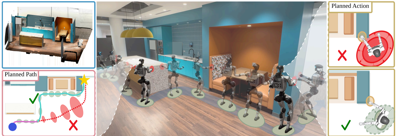
Fig. 1: TAPNAV enables vision-denied humanoid navigation through tactile active perception. The humanoid actively makes contact with the surrounding environment at informative locations, using contact observations to reduce localization uncertainty and achieve reliable navigation.
